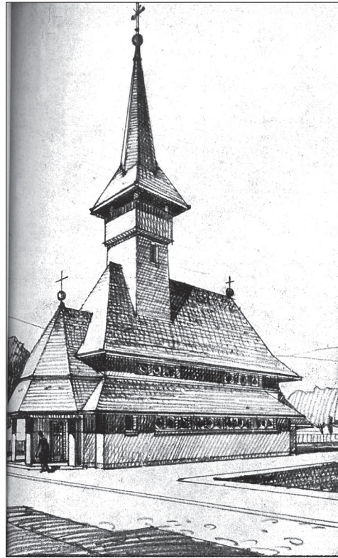
Figure 4 Petre Antonescu's proposal for the structural refinement of the massing of a wooden church in a mountainous region through the use of reinforced concrete
