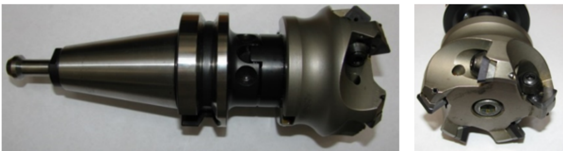
Figure 1. The applied milling head with the holder
