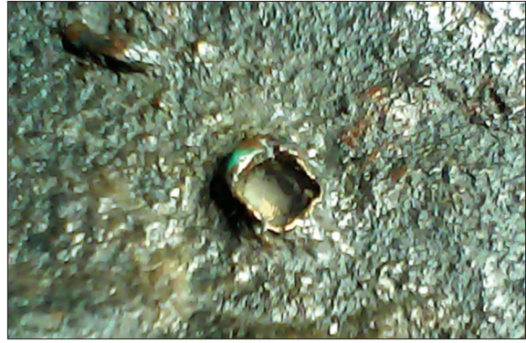
Fig. 3. Detail of spacer nail hole in the internal side of the arm.
