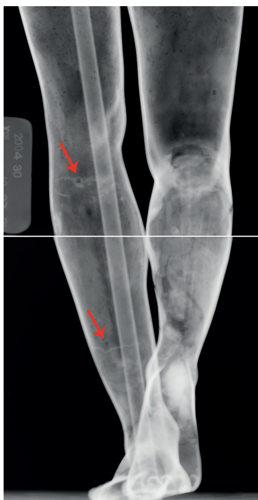
Fig. 11. Arrows indicate where two square chaplet holes are visible on the right leg in radiographs, with associated white rings of flashing.
