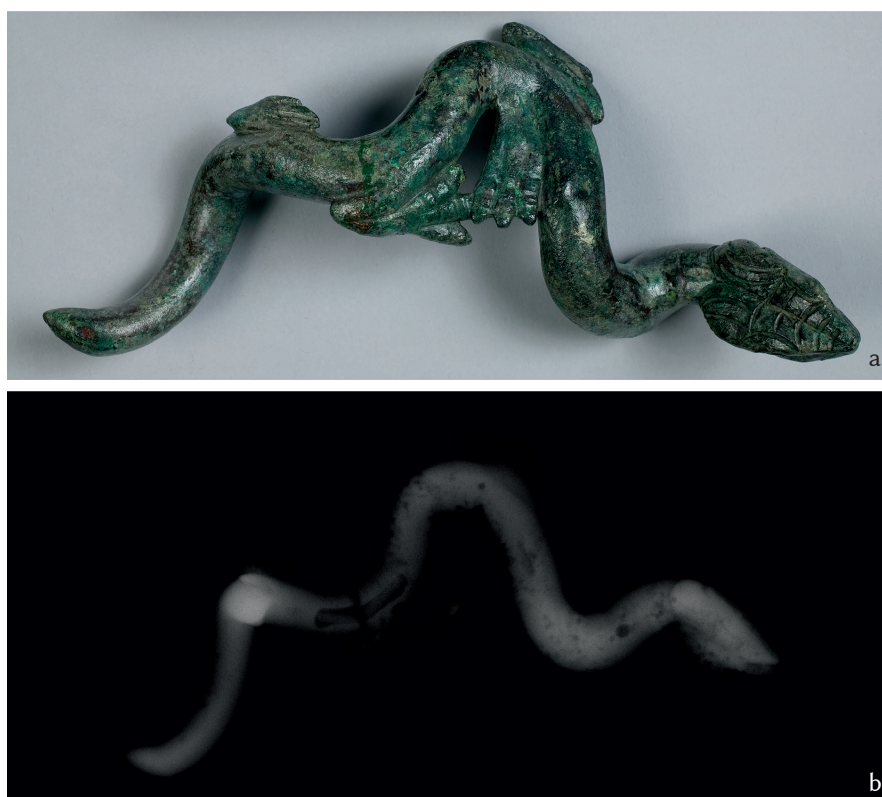
Fig. 17. A line of modern green epoxy bisects the creature at the point of the third leg (a) (Photography by Joan Neubecker). The radiograph (b) shows the metal pin repair and the more porous front half of the casting.
