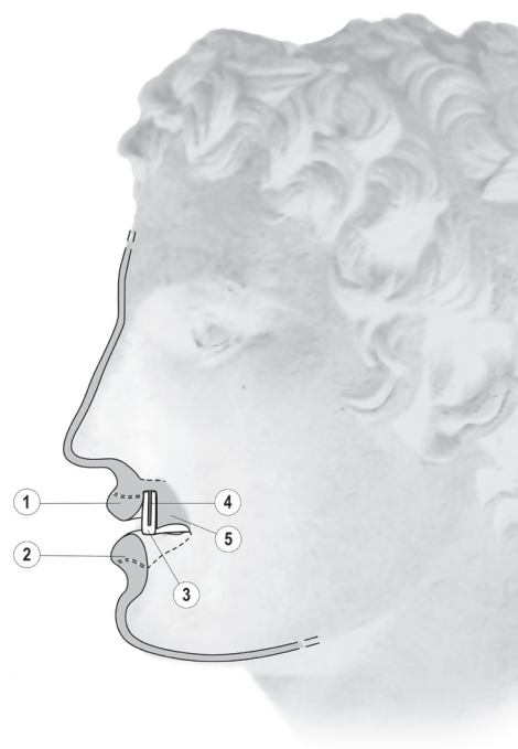
Fig. 17. Installation of teeth in large bronzes. Variant 4: teeth installed with pins in front of a tooth backplate made of bronze, 1 – upper lip, 2 – lower lip, 3 – row of teeth made of bone or ivory, 4 – mounting pins, 5 – tooth backplate (D. Greinert, Staatliche Museen zu Berlin, Museum für Vor- und Frühgeschichte).
