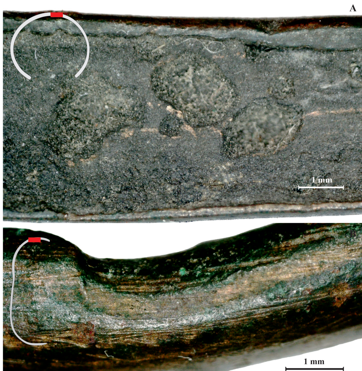
Fig. 9. Macroscopic observations. A – Shrinkage (bracelet, No. 19), B – Incomplete defect (bracelet, No. 21) (Micrographs: J. G. Tarbay)
