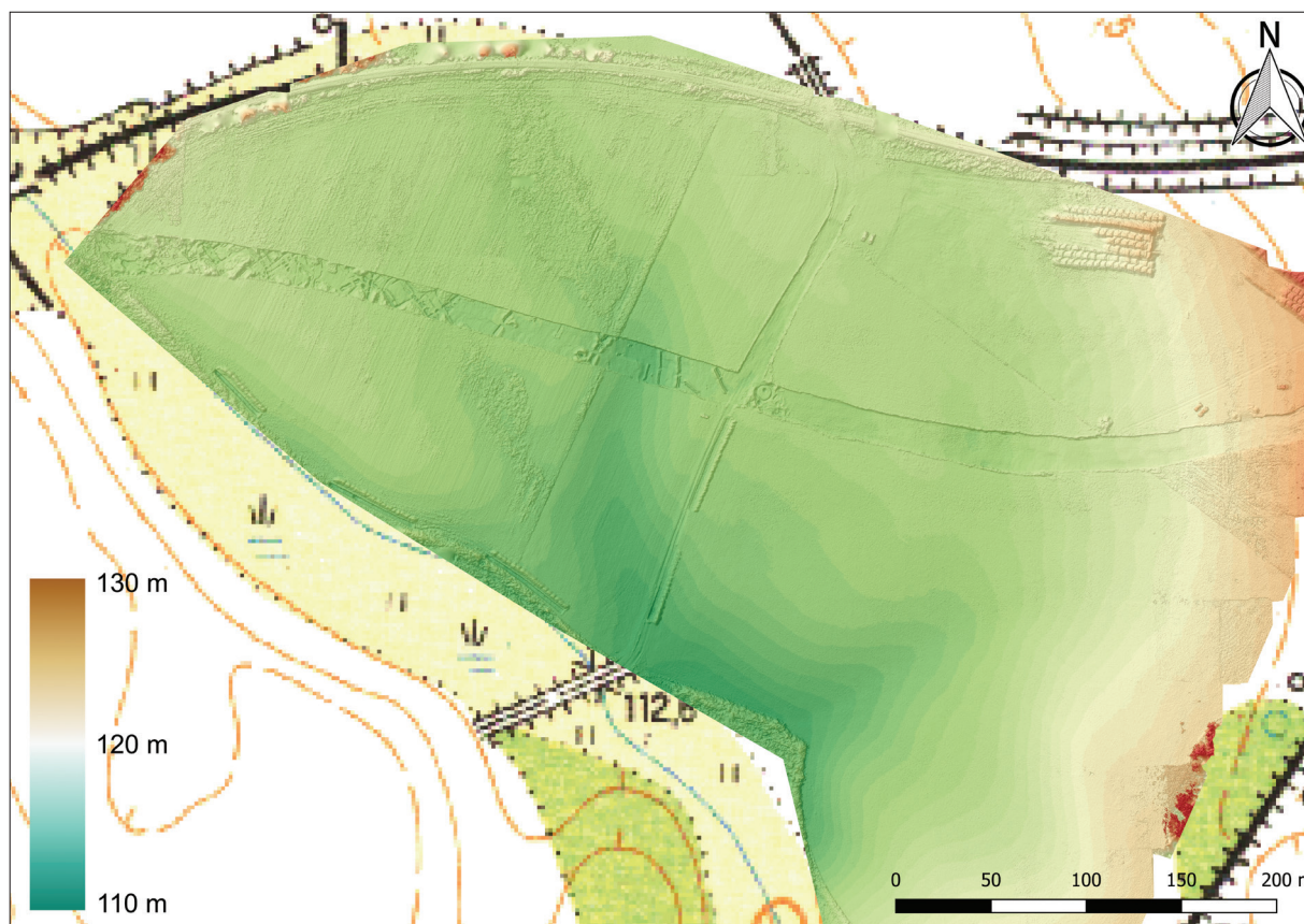
Fig. 5. The Digital Surface Modell (DSM) of the site (graphic: L. Rupnik).
