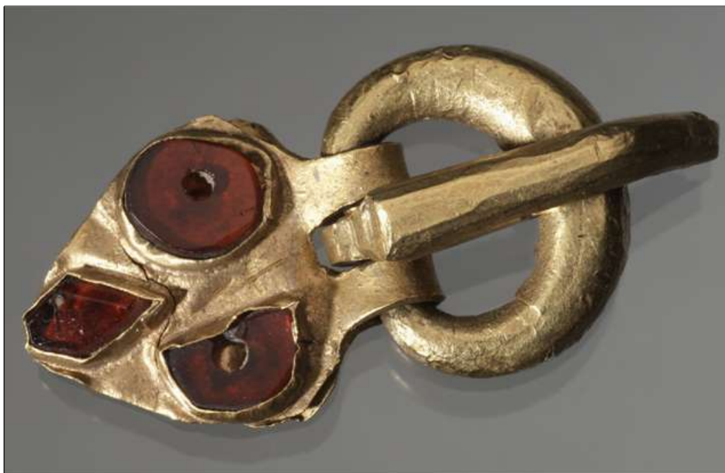
Fig. 15. Gold buckle from the Carpathian Basin made by recycling of several different objects. Plate: Au 99%, Ag 0.7%, Cu 0.2%; Tongue: Au 85%, Ag 14%, Cu 1.1%; Loop: Au 91%, Ag 8.1%, Cu 1.2% (CRADDOCK ET AL. 2010, table 1; Photo: © Trustees of the British Museum).
