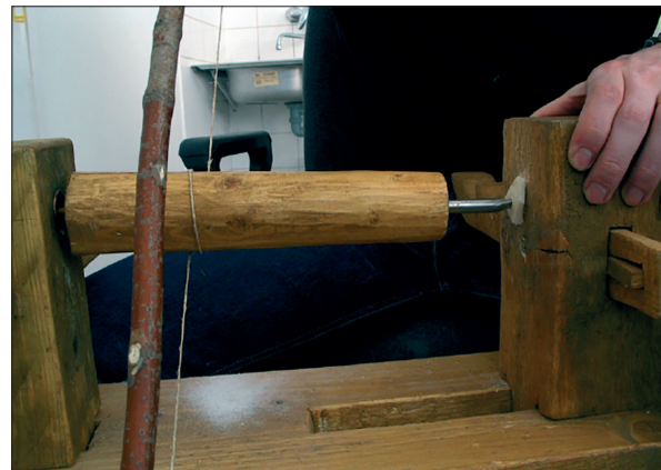
Fig. 11. The lathe used as a drill (object made by Ádám Vecsey, based on T. Bíró et al. 2012, Fig. 52).
