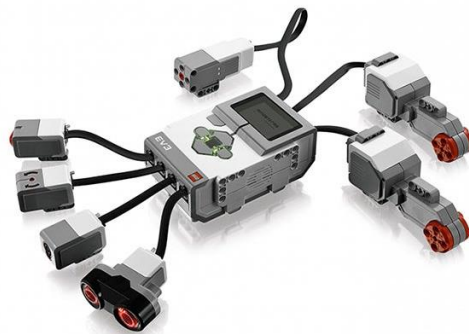
Figure 4: Options for plugging sensors and motors on a microcontroller EV3 [18]
