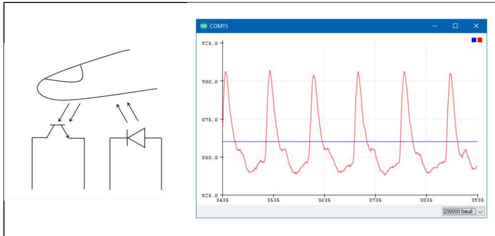
Figure 6. On the left-hand side, the arrangement of the finger photoplethysmography is shown. The plot on the right-hand side shows the Arduino's Serial plotter display of the phototransistors' output signal.
