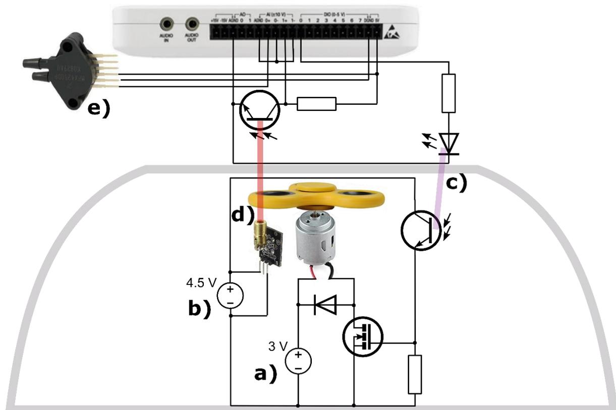
**Figure 3:** Wiring diagram of the circuits connected to the NI myDAQ device. In the lower and upper half of the figure, the circuit inside and outside the vacuum chamber is shown, respectively<sup>2</sup>
