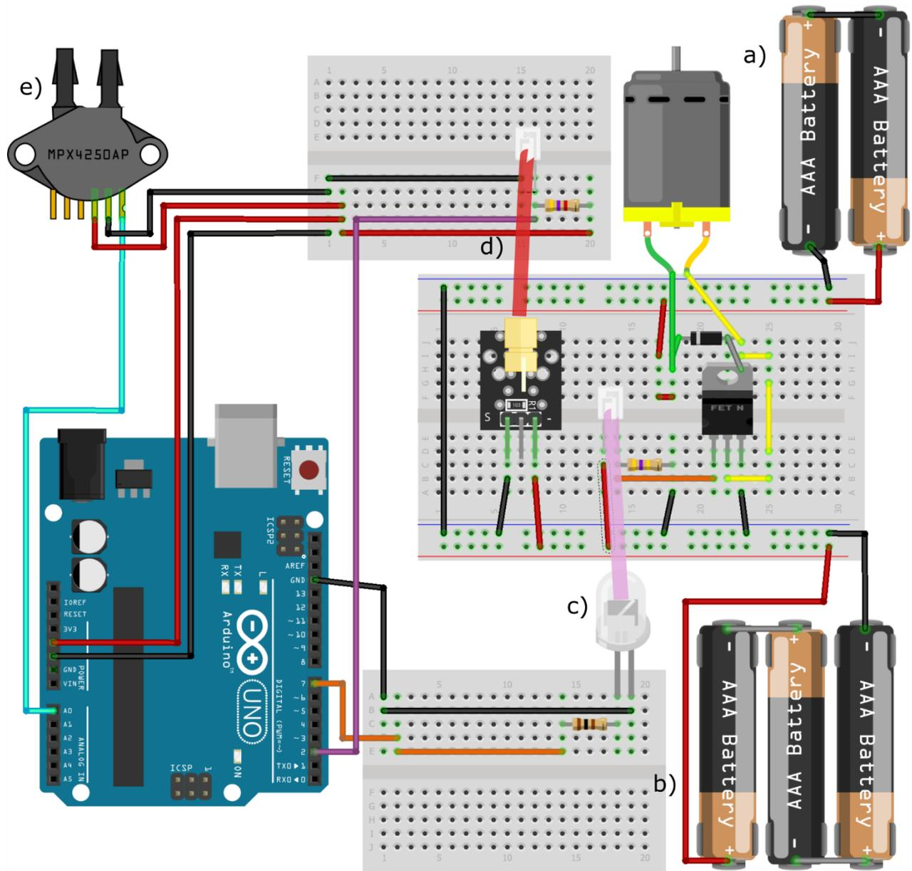
Figure 4: Building of circuits connected to an Arduino UNO on breadboards<sup>3</sup>
