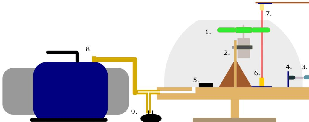
**Figure 1.a:** Structure of the measurement setup. Legend: 1. fidget spinner, 2. DC motor mounted on a stand, 3. infrared transmitter circuit, 4. infrared receiver circuit, 5. batteries 6. laser diode module 7. phototransistor circuit (6 - 7. combined: photogate), 8. vacuum pump, 9. pressure sensor<sup>1</sup>
